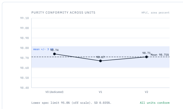
Figure 4. Purity conformity across tested units with mean and plus or minus 3 SD control band (SD 0.035%).
