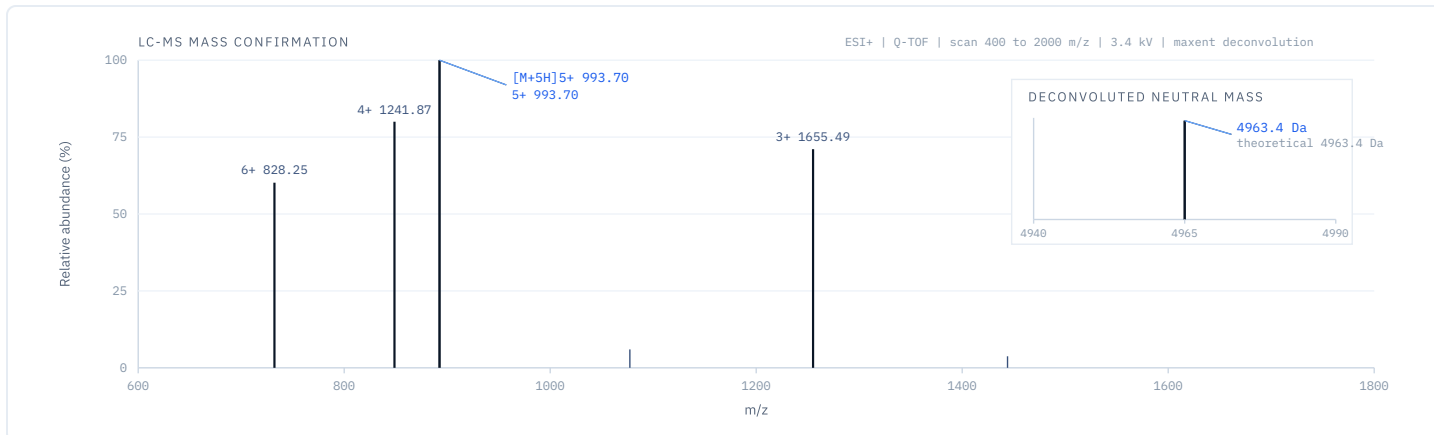
Figure 3. LC-MS mass confirmation (electrospray positive mode). The multiply-charged ion envelope from [M+3H] 3+ to [M+6H] 6+ deconvolutes to a neutral mass of 4963.4 Da, matching the theoretical mass of thymosin beta-4 (TB-500) and confirming identity.
