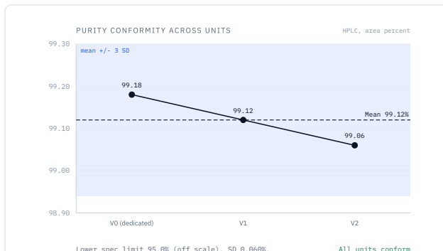
Figure 4. Purity conformity across tested units with mean and plus or minus 3 SD control band (SD 0.060%).
