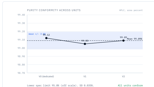
Figure 4. Purity conformity across tested units with mean and plus or minus 3 SD control band (SD 0.035%).
