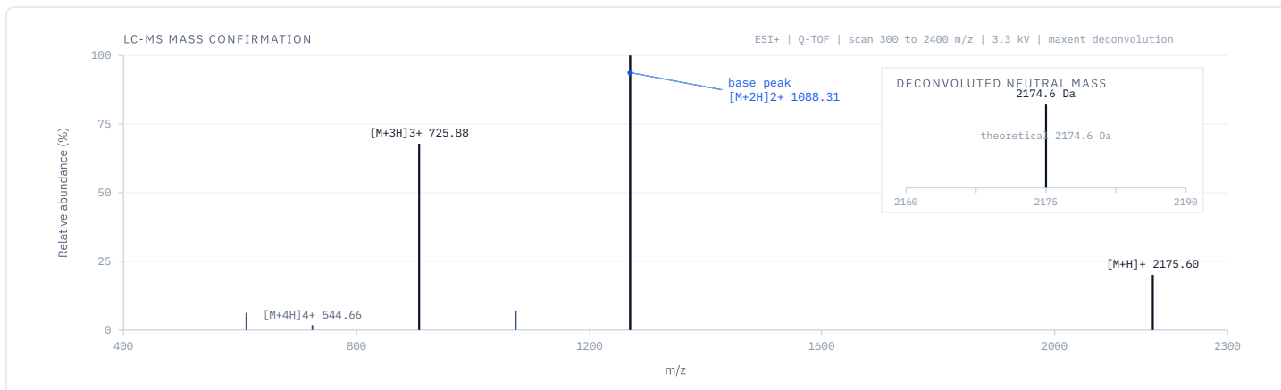
Figure 3. LC-MS mass confirmation (electrospray positive mode). Base peak [M+2H]2+ at m/z 1088.31 with the [M+3H]3+ and [M+4H]4+ ions deconvoluting to a neutral mass of 2174.6 Da, matching the theoretical mass of MOTS-c and confirming identity.
