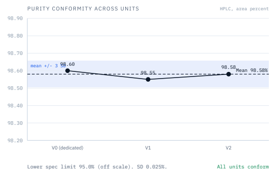
Figure 4. Purity conformity across tested units with mean and plus or minus 3 SD control band (SD 0.025%).
