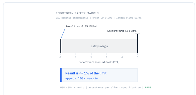
Figure 7. Bacterial endotoxin safety margin (USP <85>). Result at or below 0.05 EU/mL against a 5 EU/mL limit.
